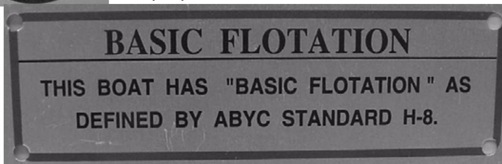
This label means that Grady-White has designed and built your boat to the ABYC standard H-8, buoyancy in the event of swamping. Basic flotation is defined as having enough foam in the boat to create buoyancy and prevent sinking under swamped conditions.
